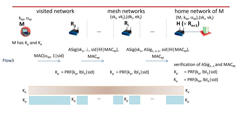
M obtains access to H over the wireless multi-hop path R<sub>1</sub>, ..., R<sub>n</sub>
